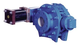
In 1991 Pratt introduced a metal seated ball valve to the municipal water and wastewater marketplace. The Pratt ball valve offers high flow rates, protected seating areas when in the open and closed position, and the ability to operate in the presence of solids and other contamination. It meets or exceeds AWWA C507 standard, has a relatively low torque for operation, and has a long life in high-cycle conditions. Pratt's ball valve passed the 10,000 cycle test.
