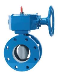
Pratt's 2FII™ rubber seated butterfly valves are available in sizes 3" through 20". The shafts are constructed of center-less, ground ASTM A276 type 304 or 316 stainless steel bar and thus are not susceptible to corrosion as are carbon steel or other similar materials. Shafts are
