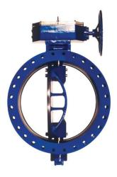
The Pratt Triton™ Butterfly Valve has a rubber seat located in the body that reduces performance problems related to corrosive buildup in valve body and pipeline. The E-Lok seat can be adjusted and/or repaired in the field without dewatering the pipeline or removing the valve from the line. The flow through
