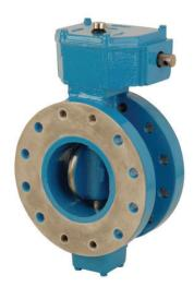
Henry Pratt now offers a 350psi, 525 shell test, ANSI 250#, Butterfly Valve - the first in the industry! This valve is excellent in high pressure applications. The valve body and disc are made of ductile iron with the rubber seat in the body for abrasion resistance and bubbletight closure. Available in 6" - 48" with flanged end connections.
